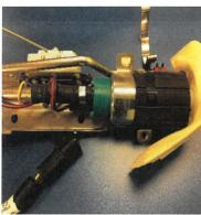
NOTE: Failure to use a new filter on the fuel pump inlet will likely result in premature pump failure and will void the pump warranty if applicable.
